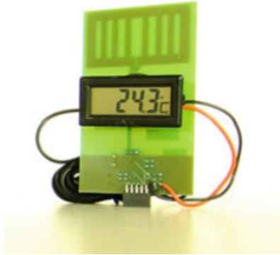
Figure 4: Rectenna integrated with temperature system operating at 915 MHz [1].
