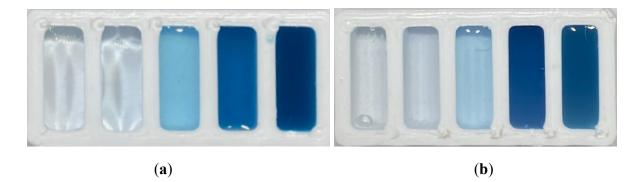
**Figure 2:** Colorimetric ladders generated by previous teams to compare sensor sensitivity. Varying concentrations of *E. coli* were induced with (a) DHBM and (b) whole bovine milk. We also used these same images to test our colorimetric algorithm.
