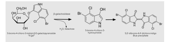
Figure 1: Reaction schematic for X-gal hydrolysis in the presence of  $\beta$ -galactosidase. The blue precipitate product is used in our assay for colorimetric analysis.
