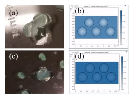
Figure 6: Comparison of experimental data and COMSOL model surface concentration outputs for blue reaction precipitate. a) Experimental after 30 mins incubation, b) COMSOL output at 30 minutes reaction time, c) Experimental after 60 mins incubation, d) COMSOL output at 60 minutes reaction time. Figure 6a and 6c from Madamba, 2019 [65].
