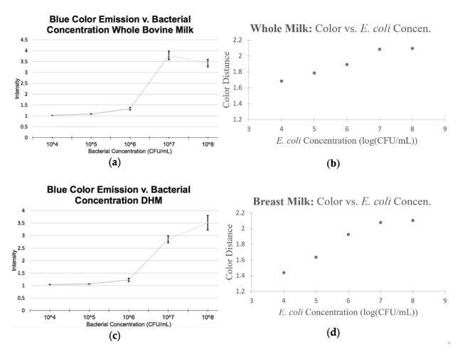
**Figure 13:** Graphs depicting the calculated color values for various concentrations of *E. coli* induced with (a) whole bovine milk, analyzed using previous algorithm, (b) whole bovine milk, analyzed using new algorithm, (c) DHBM, analyzed using previous algorithm, (d) DHBM, analyzed using new algorithm. Analysis performed on the same set of image data obtained from previous MilkGuard Team's laboratory results.
