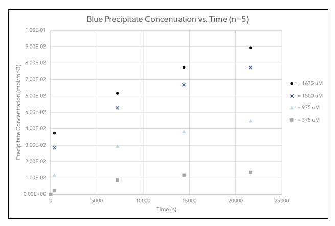
**Figure 8:** Reaction precipitate concentration over time for capsules of selected radii. Results indicate that greater total capsule volumes produce more rapid results.
