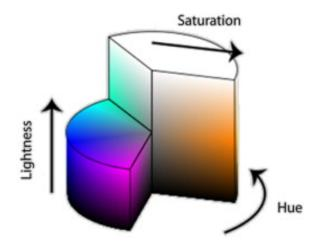
**Figure 5:** An HSL color cylinder model showing the corresponding dimensions for Hue, Saturation, and Lightness [56].
