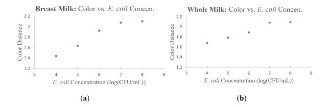
**Figure 10:** Graphs depicting the calculated Color Distance Values for various concentrations of *E. coli* induced with (a) DHBM and (b) whole bovine milk. Image data obtained from previous MilkGuard Team's laboratory results.
