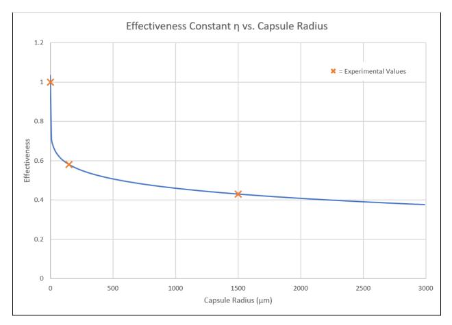
Figure 4: Effectiveness constant as a function of capsule radius, from experimentally derived values.
