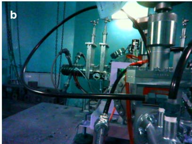
Fig. 5 (a) Normal web camera image. (b) Green on web camera disappears due to neutron irradiation.
