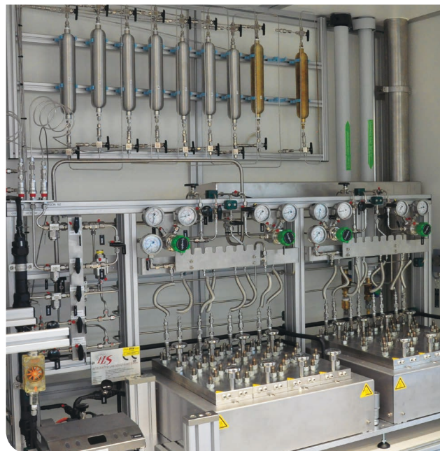
Set-up for high-throughput catalyst screening (photo Christophe Copéret, ETH)
