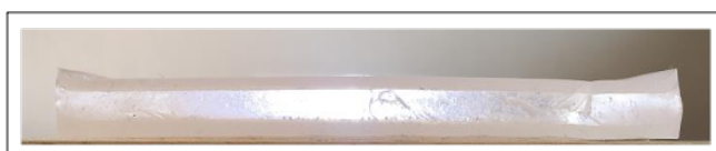
Figure 4: Detailed structure of the mimicking Subcutis layer consisting of EG layer (illuminated) wrapped in 2 DS layers.
