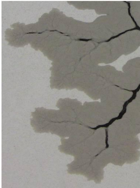
Figure 46: Micro-fractures forming between the sand layer and Hele-Shaw cell. Test A4
