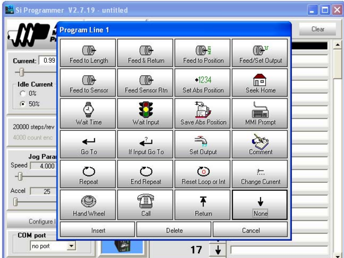
Figure 4-6: Screenshot from the SI programmer software. This picture depicts the main programming interface in the background with all the potential controls over the linear actuator in the foreground.
