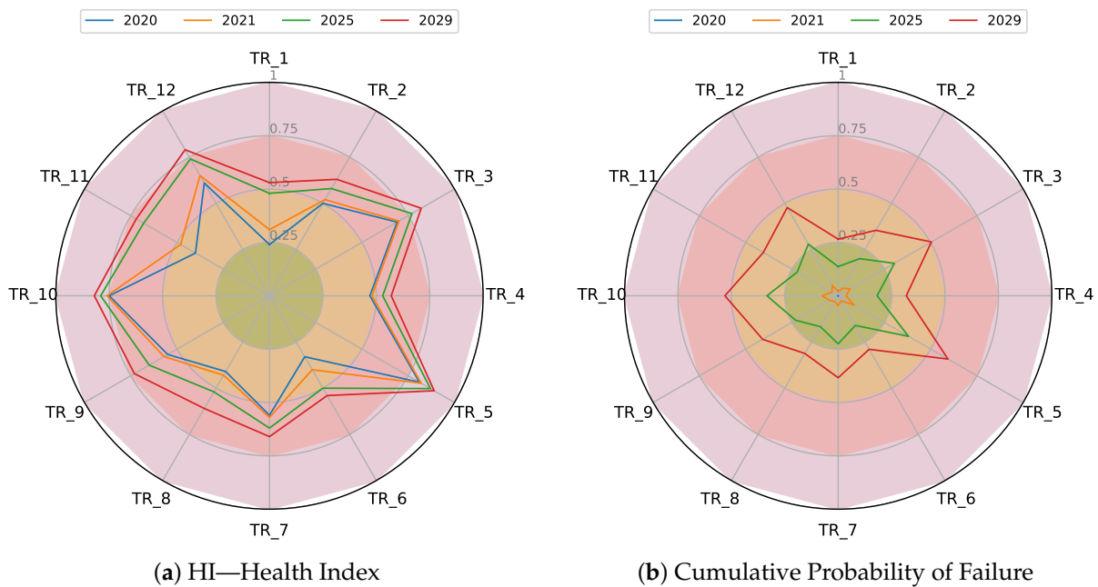
Figure 7. Health index prediction and cumulative probability forecast of failure for the transformer fleet.
