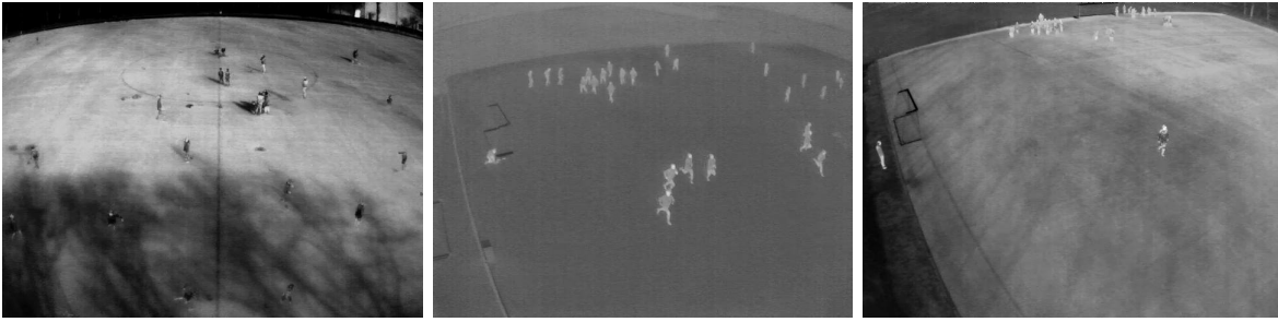
Fig. 1. Person representation in thermal images (a) Person appeared darker w.r.t background, (b) Person appeared lighter w.r.t background, (c) Person appeared similar to background
