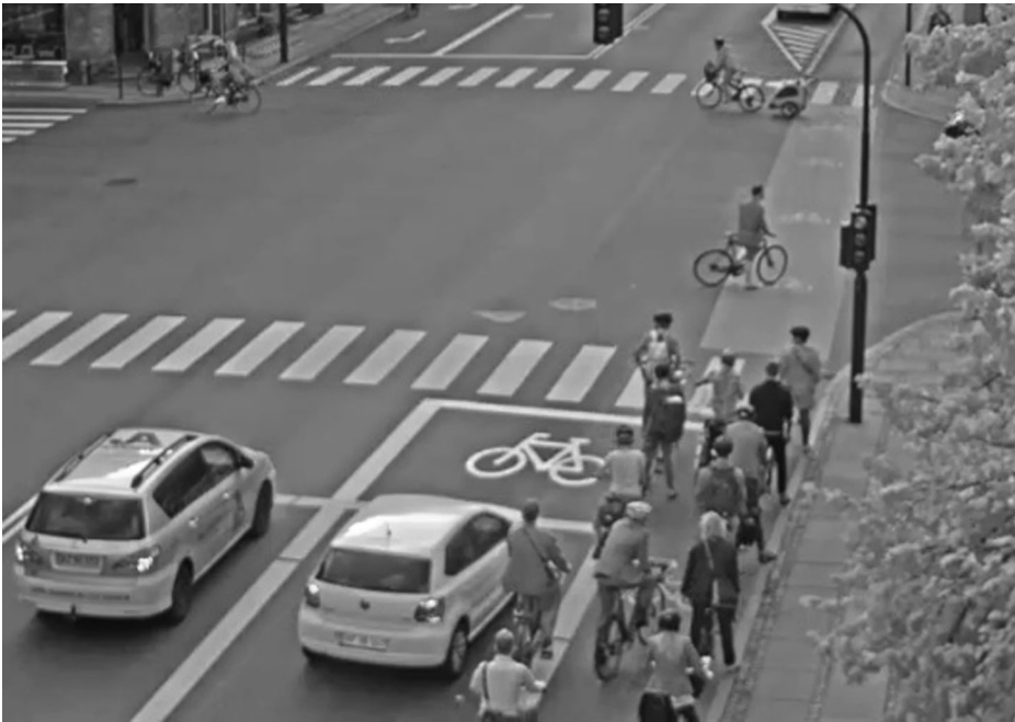
Figure 8. ASB not in use. Cyclists in the front block the entry to the ASB for the other cyclists.
