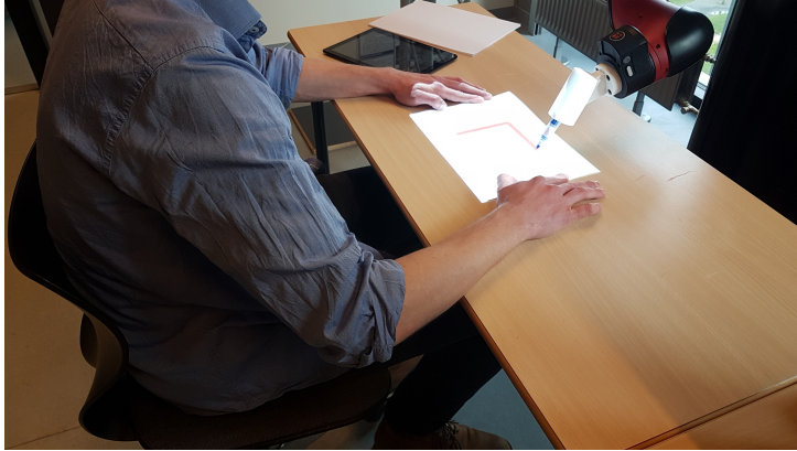
Fig. E.4: A participant sitting in front of the robot, holding the paper down. The paper is held in the area marked with a projected white rectangle, fitting an A4 sheet of paper. The robots holds the felt pen in a custom-designed 3D printed mount that is fitted with foam. The robot draws along the red line which is projected on the paper. To the participant's left is the stack of paper they can grab from and the tablet used to answer the questionnaire throughout the test.
