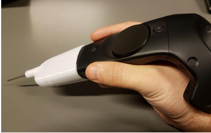
Fig. B.5: The needle used for the experiment, made from a 3D printed mount and a nail attached with a bolt in the loop designed for the wrist strap.
