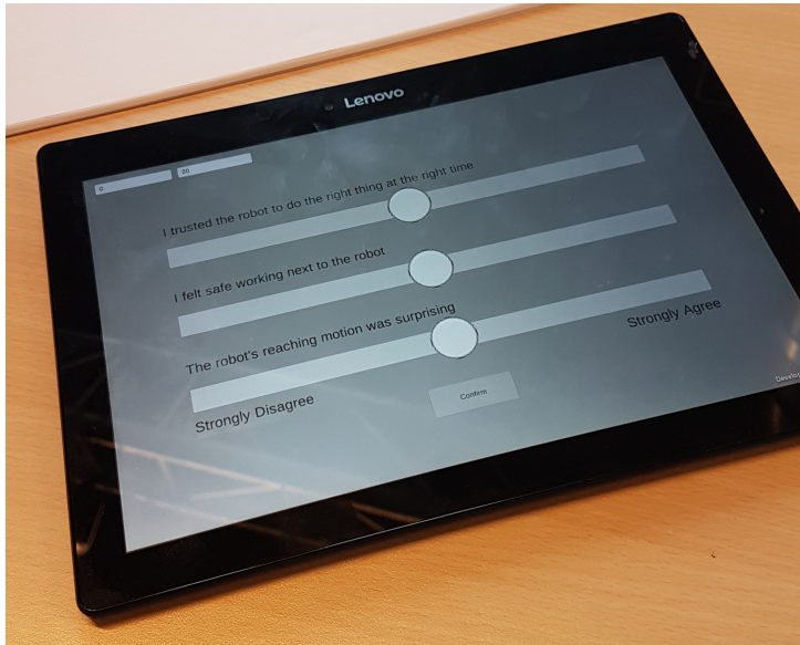
Fig. 4.1: The tablet used to administer the short trust scale questionnaire. The sliding scales let the participants quickly report their attitude toward the robot as level of agreement with the three statements [1]
