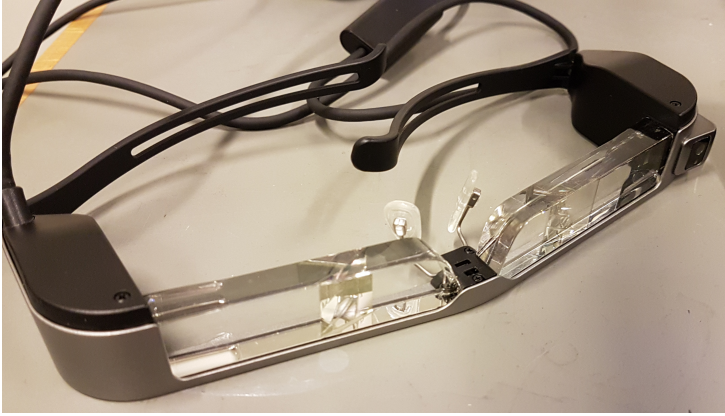
Fig. B.1: The Epson Moverio Bt-300 glasses used for the experiment. [2]
