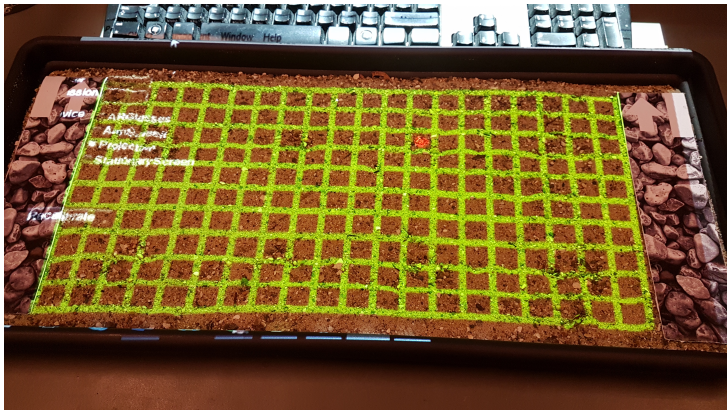
Fig. B.3: The grid projected onto the sand with the targets shown as a red dot. [2]
