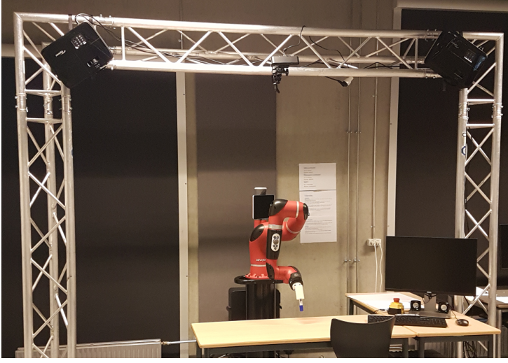
Fig. E.1: Full HRC cell setup with Sawyer robot, projectors and infrared camera.
