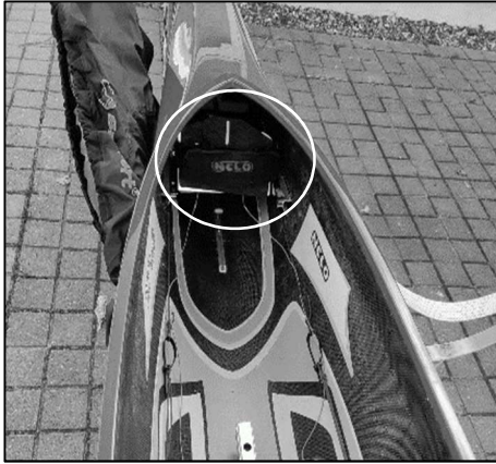
Figure 9: The footrest mounted in a kayak. Adapted from Study II.
