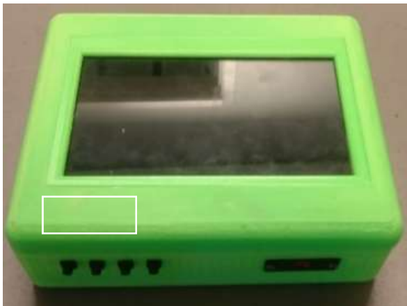
Figure 11: Portable custom-built data acquisition system in the waterproof casing. Note the four input binder connectors in the bottom left portion of the photograph.
