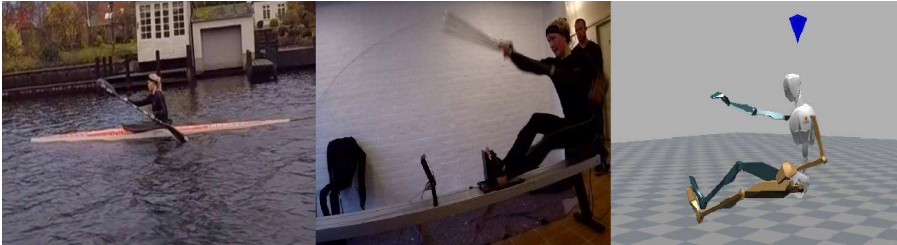
Figure 6: View of the on-water test, the on-ergometer test (B), and the Xsens 3D representation of an ergometer test.
