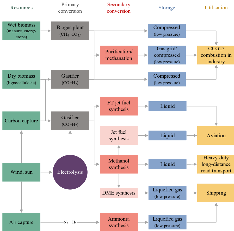
Figure 13: The four pathways for renewable fuel production in a system perspective.
