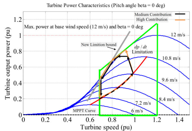
FIGURE 3. The proposed Inertia control process of a wind turbine with the defined limitations.
