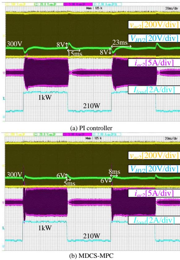
Fig. 21. Transition waveforms under V_{HV1}=300V , V_{HV2\_ref}=300V
