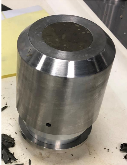
Fig. 8. Sample preparation of Søvind Marl in the oedometer ring.
