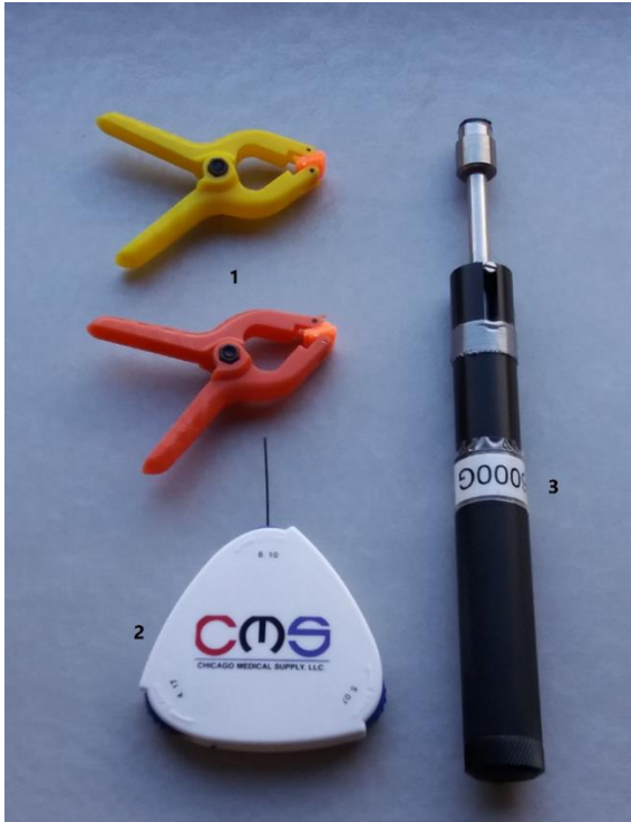
Figure 7: Illustration of the bed-side tools used for the quantitative sensory profiling of pain sensitization. 1: Standard clamps. 2: Nylon filament. 3: Spring-based pressure- algometer.
