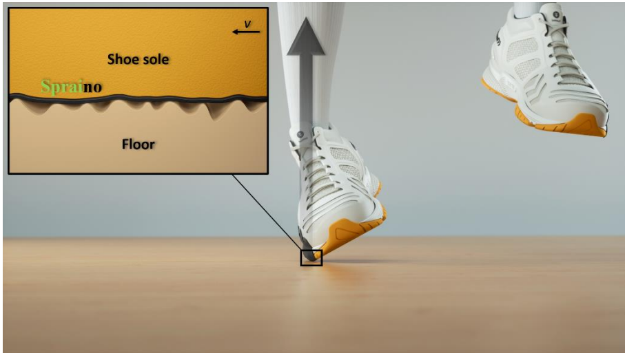
Figure 4-3. Low shoe-surface friction during a bad landing due to Spraino. Adapted with permission from Lysdal et al. (94)
