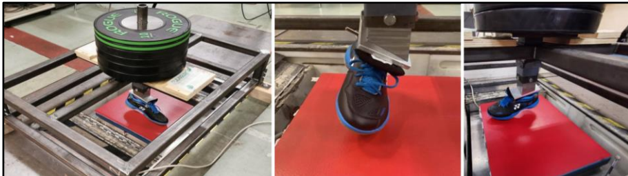
Figure 4-4. Mechanical setup of the modified ISO: 13287:2019 slip resistance test. Shoe is fixed in 15° pitch and 30° roll angle in relation to the floor surface and loaded with 50 kg.
