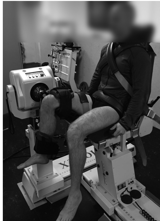
Figure 2: The picture illustrates the experimental set-up using the Biodex. The participant was comfortably seated with the trunk and lower extremities securely fastened with straps. The lever arm of the Biodex passively moved the lower leg towards extension at a speed of 5^\circ/\text{s} .
