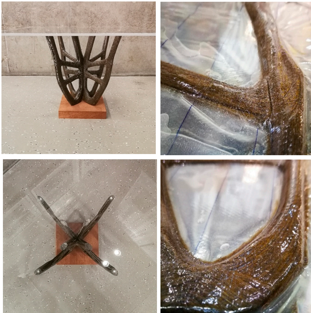
Figure 11. Shape and laminate composition of the structure, close-up of the surface characteristics (counterclockwise from top left to bottom right).
