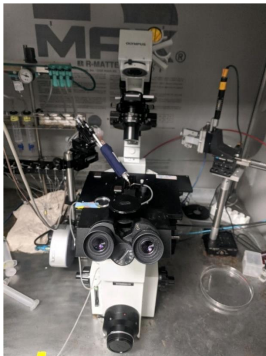
Figure 29. Photo of the fluorescent microscope used to acquire functional data of compounds at 5-HT 2B receptors.
