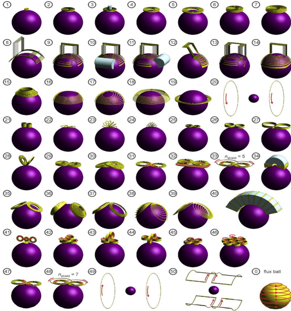
Figure 6: Simulation models of 50 TMS coil configurations: (1) Animal mini-coil, (2) Magstim 50 mm circular coil (P/N 9999), (3) 50 mm circular coil with iron core, (4) Magstim 70 mm circular coil (P/N 3192), (5) Magstim 90 mm circular coil (P/N 3192), (6) Magstim animal MST coil, (7) Magstim human MST coil (S/N MP39), (8) Brainsway H coil, (9) Brainsway H1 coil, (10) H1 coil with frontal iron core, (11) H1 coil with lateral iron core, (12) Brainsway H1L coil, (13) Brainsway H2 coil, (14) Brainsway HADD coil, (15) Magstim cap coil, (16) crown coil, (17) crown coil with back-splayed winding, (18) crown coil with back-spaced winding, (19) supraorbital halo coil, (20) MRI z-gradient coil in parallel-current (Helmholtz) mode, (21) 3-layer double coil, (22) double butterfly, (23) circular slinky-7 coil, (24) rectangular slinky-7 coil, (25) Magstim 25 mm figure-8 (P/N 1165), (26) Cadwell Corticoil, (27) Cadwell B-shaped coil, (28) 50 mm V-coil, (29) MagVenture C-B65 butterfly coil, (30) MagVenture MC-B70 butterfly coil, (31) Magstim 70 mm figure-8 coil (P/N 9925, 3190), (32) 70 mm figure-8 with shielding plate, (33) 70 mm figure-8 with active shield (5 turns), (34) Neuronetics iron core figure-8 coil (CRS 2100), (35) MagVenture D-B80 butterfly coil, (36) MagVenture MST twin coil, (37) Magstim double cone coil (P/N 9902), (38) eccentric double cone coil with center-dense windings, (39) eccentric double cone coil with center-sparse windings, (40) stretched C-core coil, (41) 3-D differential coil, (42) 3-D coil array #1, (43) 3-D coil array #2, (44) 3-D coil array #3, (45) Cadwell cloverleaf coil, (46) circular coil array, (47) Magstim 70 mm figure-8 coil in reversed-current mode, (48) 70 mm figure-8 with active shield (7 turns), (49) MRI z-gradient coil opposing-current (Maxwell) mode, and (50) MRI x- (or y-) gradient (Golay) coil. The last configuration,
