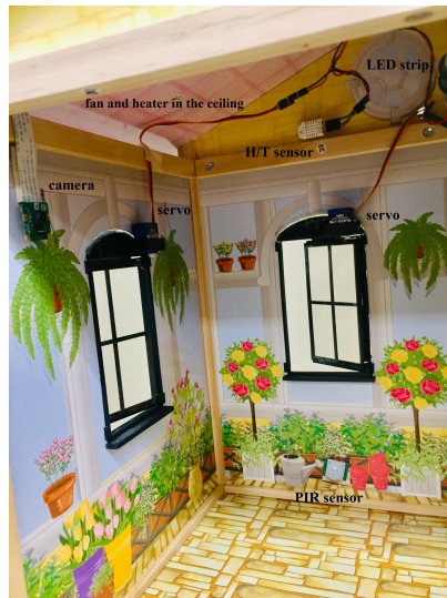
Figure 3.10: Picture of one room including its actuators and sensors
