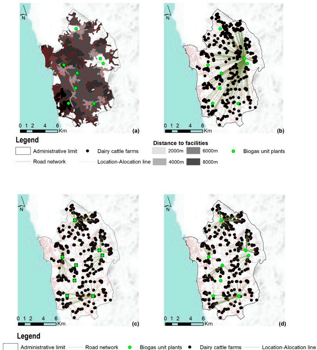
Figure 5. (a) Distance road analysis (m) to biogas plants; (b) Allocation analysis considering centralized (1 biogas facility); (c,d) distributed scenarios (5 and 8 facilities).
