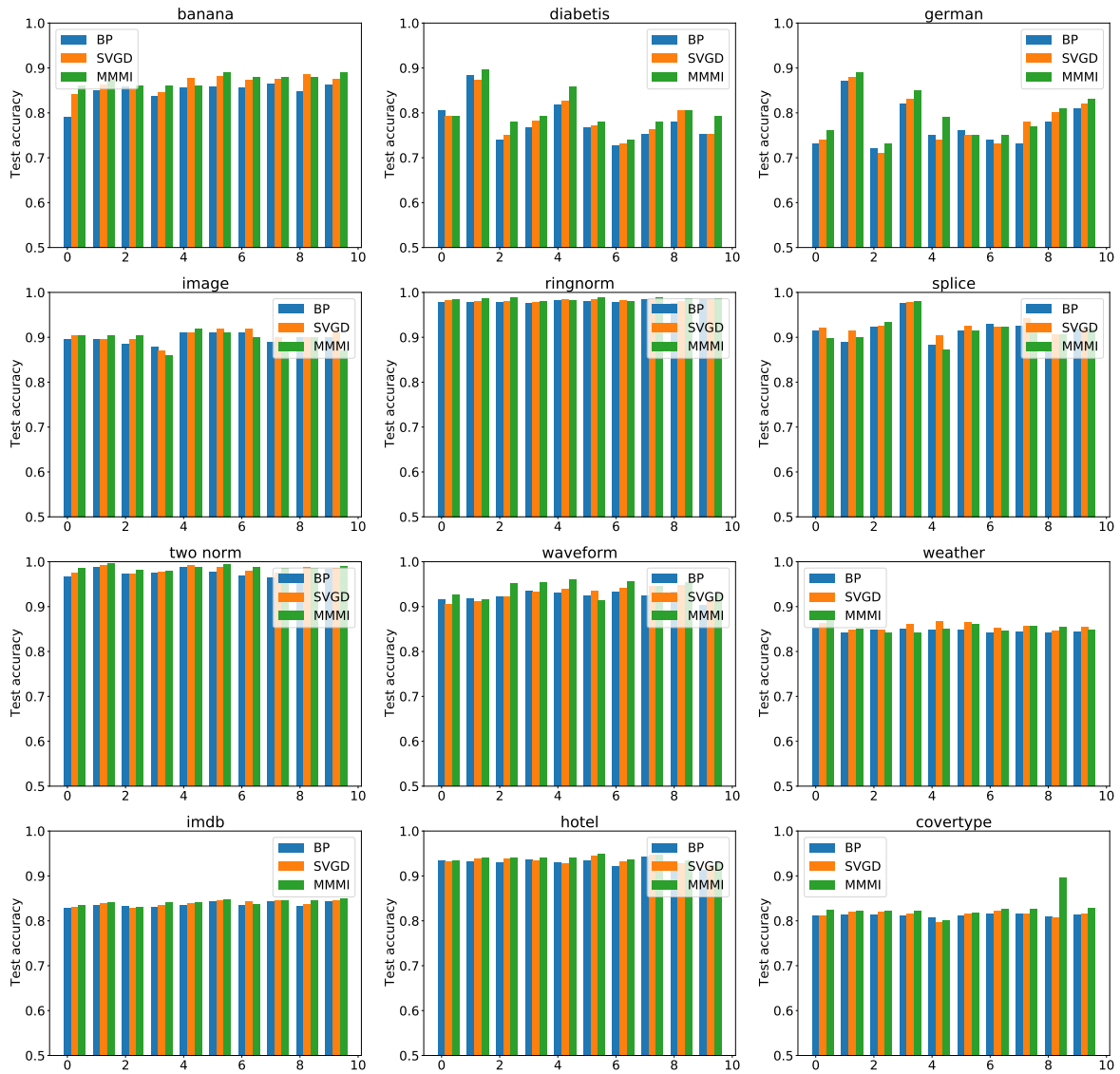
Figure 4.5: Test accuracy of BP, SVGD, MMMI for neural networks on 12 datasets over 10 random seeds
