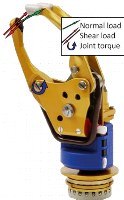
Figure 5 View of the Ottobock SensorHand Speed system without silicone cover, integrated sensory suite illustrated.
