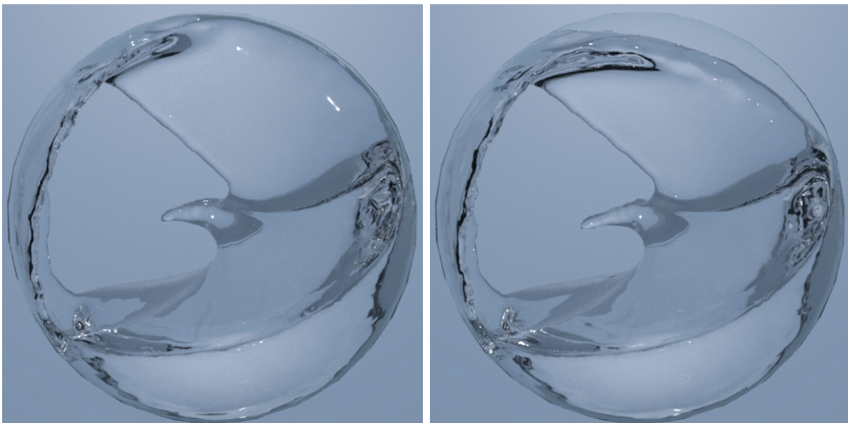
Figure 3.1: A selected frame from two simulations of a 3D scenario of fluid splashing inside a spherical boundary. Left: Without separating solid wall boundary conditions, the fluid adheres to the top of the sphere. Right: With separating solid wall boundary conditions, the fluid separates naturally.
