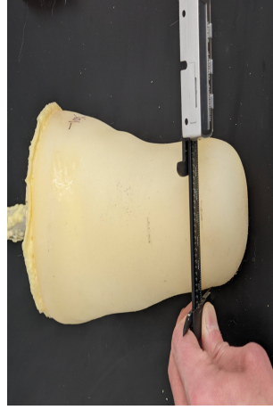
Figure 14: Measurement method for in vivo measurements for biofidelic limbs
