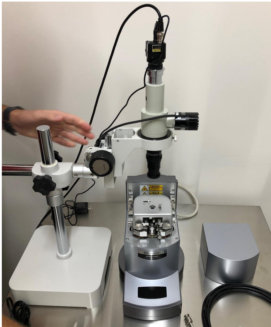
Figure 25: Shimadzu's SPM 9700-HT used for topographical observations and KFM analysis. SPM was carried out on specimens grown on 12.7 x 12.7 mm corning glass substrates with evaporated silver nanorod films as shown in Figure 26.
