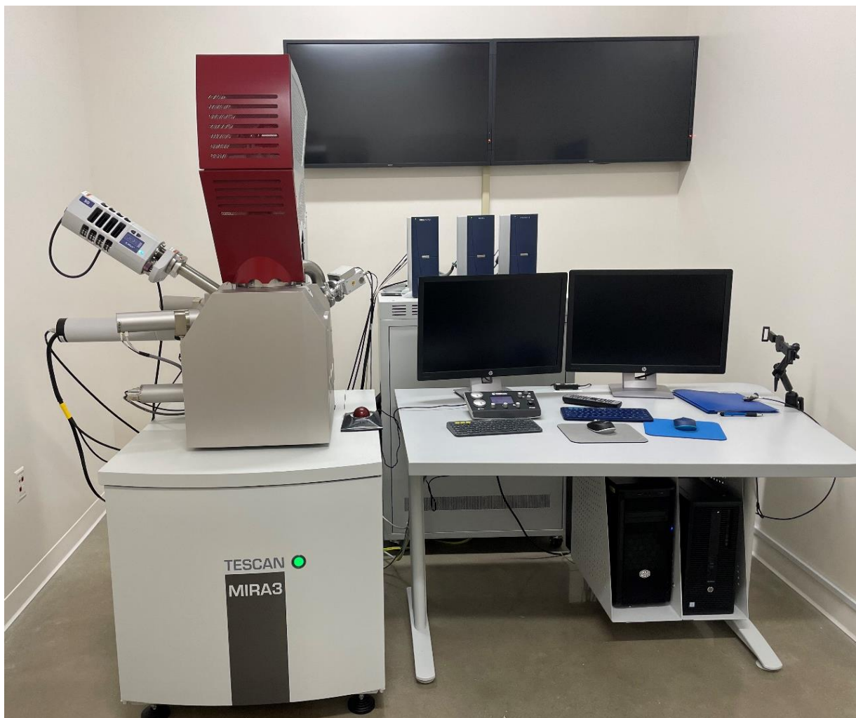
Figure 24: Tescan Mira3 SEM used to obtain sample images and EDS spectrum
