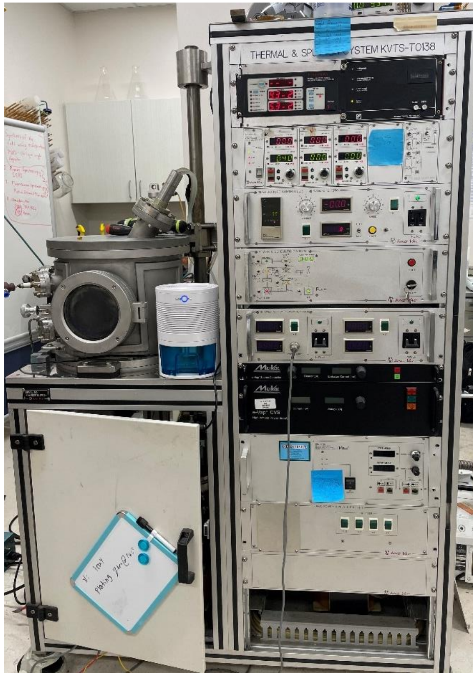
Figure 21: PVD System configuration with the custom-built high vacuum chamber on the top left
