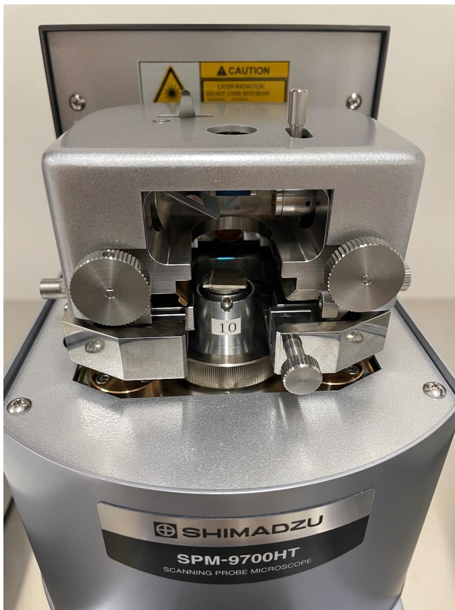
Figure 26: Ag glass sample sitting on the 10 micron scanner.
