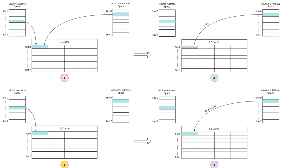
Figure 2.13: Illustration of the Flush+Reload attack by means of a 4-way (columns) cache with 8 sets (rows). In step 1, the attacker or the victim cache a shared line. In step 2, the attacker flushes the shared cache line. In step 3, the victim accesses the previously accessed cache line. In step 4, the attacker tries to reload the cache line. If the cache has been accessed by the victim, the attacker will experience a fast access time.
