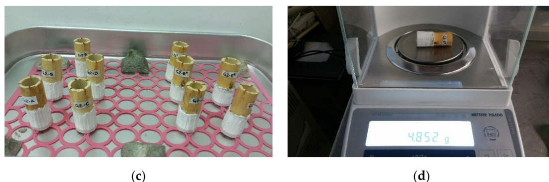
Figure 4. Capillary water absorption test steps: (a) sample preparation, (b) steel wire support, (c) samples immersed in water, and (d) weighing the sample on a precision balance.
