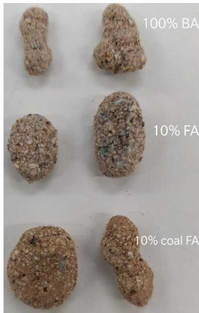
Figure 13. Elongated shapes in 800 °C sintered samples.
