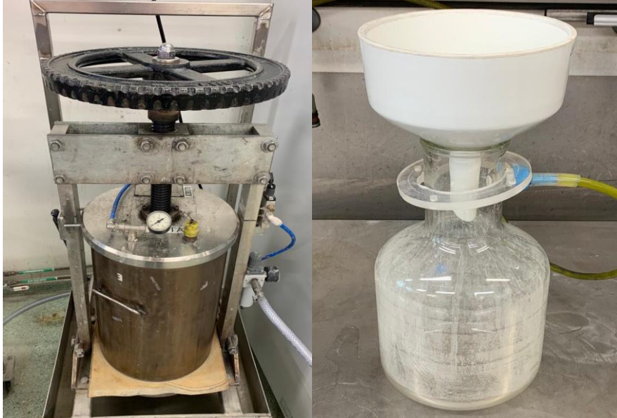
Figure 30 Pressure and vacuum filters
