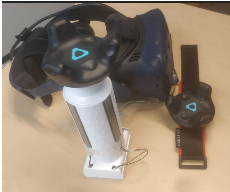
Figure 10. Experimental device consisting of prototype with FSR sensors, board and HTC VIVE Tracker (left down); strap with HTC VIVE Tracker (right); and HTC VIVE Pro 2 headset (top).
