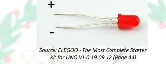
In this project, it is going to be used one green, one red and one yellow LEDs. The red and green LEDs are intended to show the status of the alarm, whether it is enabled or disabled. The yellow LED is used as an illumination light.
