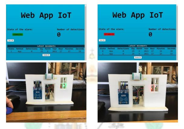
Turning on the alarm through the Web App and turning it off using the RFID tag:
