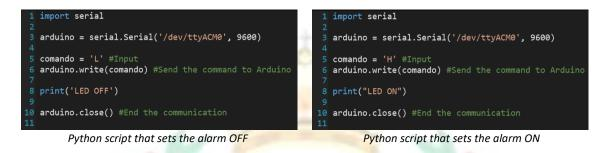
The communication from the Arduino to the Raspberry is way easier. Arduino is constantly sending the value of the state of the alarm to the Raspberry at the beginning of every loop.
