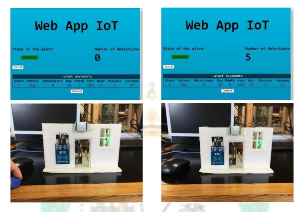
The app displays the number of movements detected in the period when the alarm is enabled. Then, when the alarm is turned off, it displays in the table how many movements were detected in that period in total.
