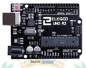
The main board of this project is the Arduino UNO. The one I used is not from the original brand *Arduino* but due to the fact that it is open source, there a lot of manufacturers that make their own. The one I have used is the **Elegoo UNO R3 Controller Board**.
