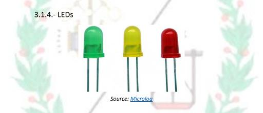
A light-emitting diode (LED) is a semiconductor light source that emits light when current flows through it. Electrons in the semiconductor recombine with electron holes, releasing energy in the form of photons. The color of the light (corresponding to the energy of the photons) is determined by the energy required for electrons to cross the band gap of the semiconductor. [15]
