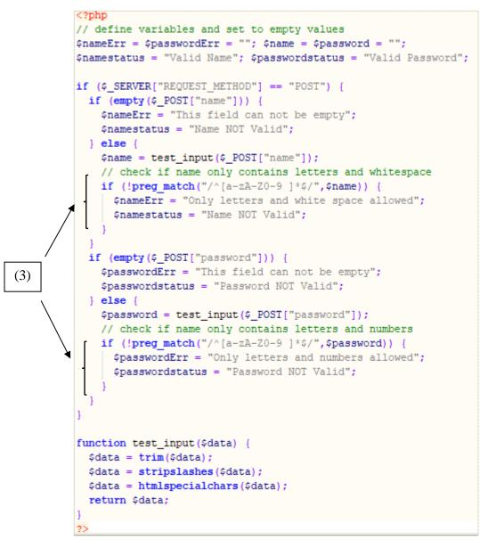
Figure 5.17: Screenshot of the main code in secure\_validation.php
