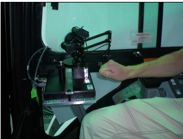
Figure 4: Sensable Phantom Premium 1.0 mounted out- and inside the cab
