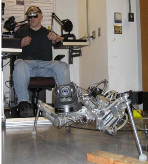
Figure 6: Operator interface and Two-legged Robot model before design revision
