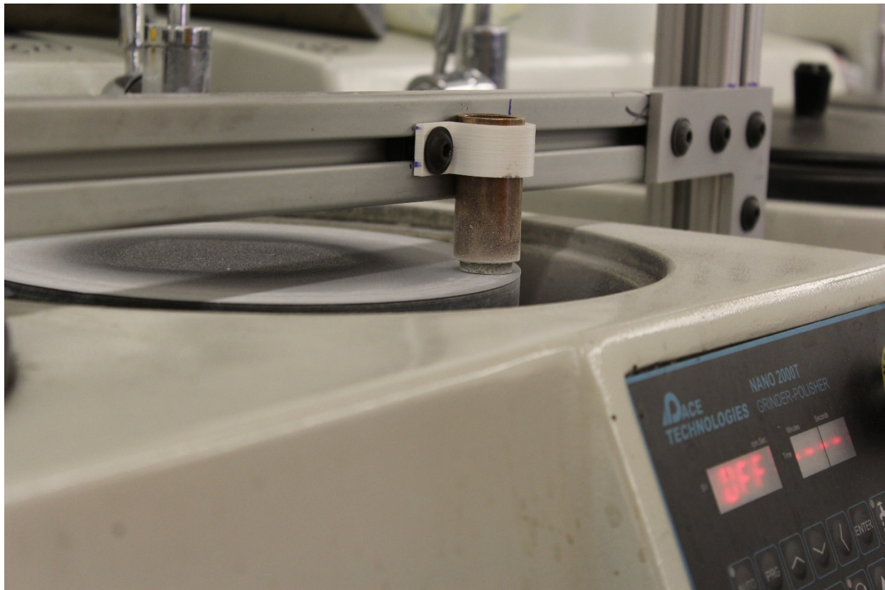
Figure 10. Accelerated Contact Surface Wear Test with GFRP
