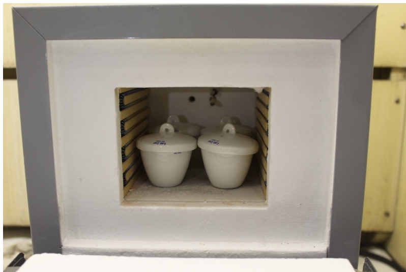
Figure 4. High Temperature Burnoff Following ASTM D 3171 – A7
