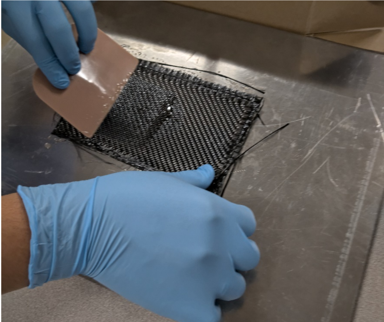
Figure 2. Traditional Wet-Layup Composite with Carbon Fibers and Epoxy Matrix
