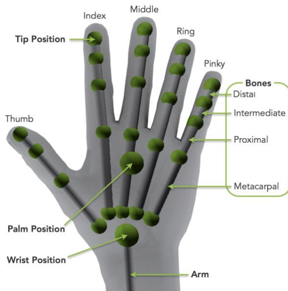
Figure 23: Hand Joint Points as seen by Leap Motion Controller[22]
