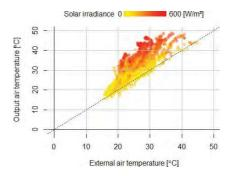
Figure 4: Inlet-outlet temperature gain in the cavity. (Roberto Garay-Martinez et Al. (2020))
