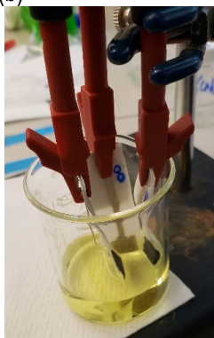
Figure 26. (a) Potentiostat and Electrochemical Characterization Test Setup (b) Textile electrodes printed on separate substrates in 0.5 M KCl solution of K_3Fe(CN)_6 ; (c) Pine Research SPE with IO Rodeo attachment in 0.5 M KCl solution of K_3Fe(CN)_6
