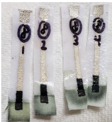
Figure 23. Drop-cast PANI onto textile WE
