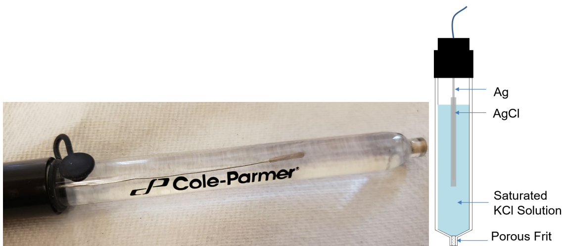
Figure 5. Standard Ag/AgCl RE
