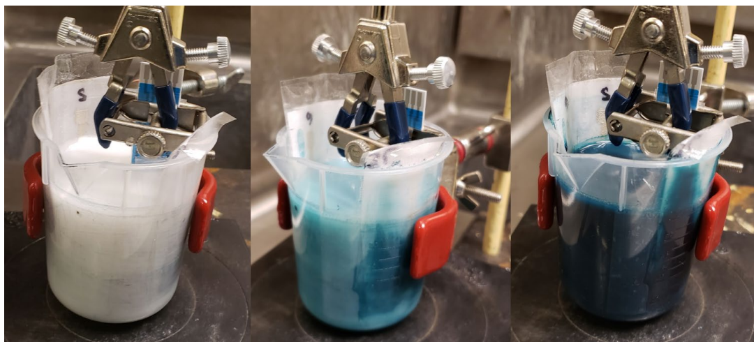
Figure 17. PANI chemical polymerization progression
