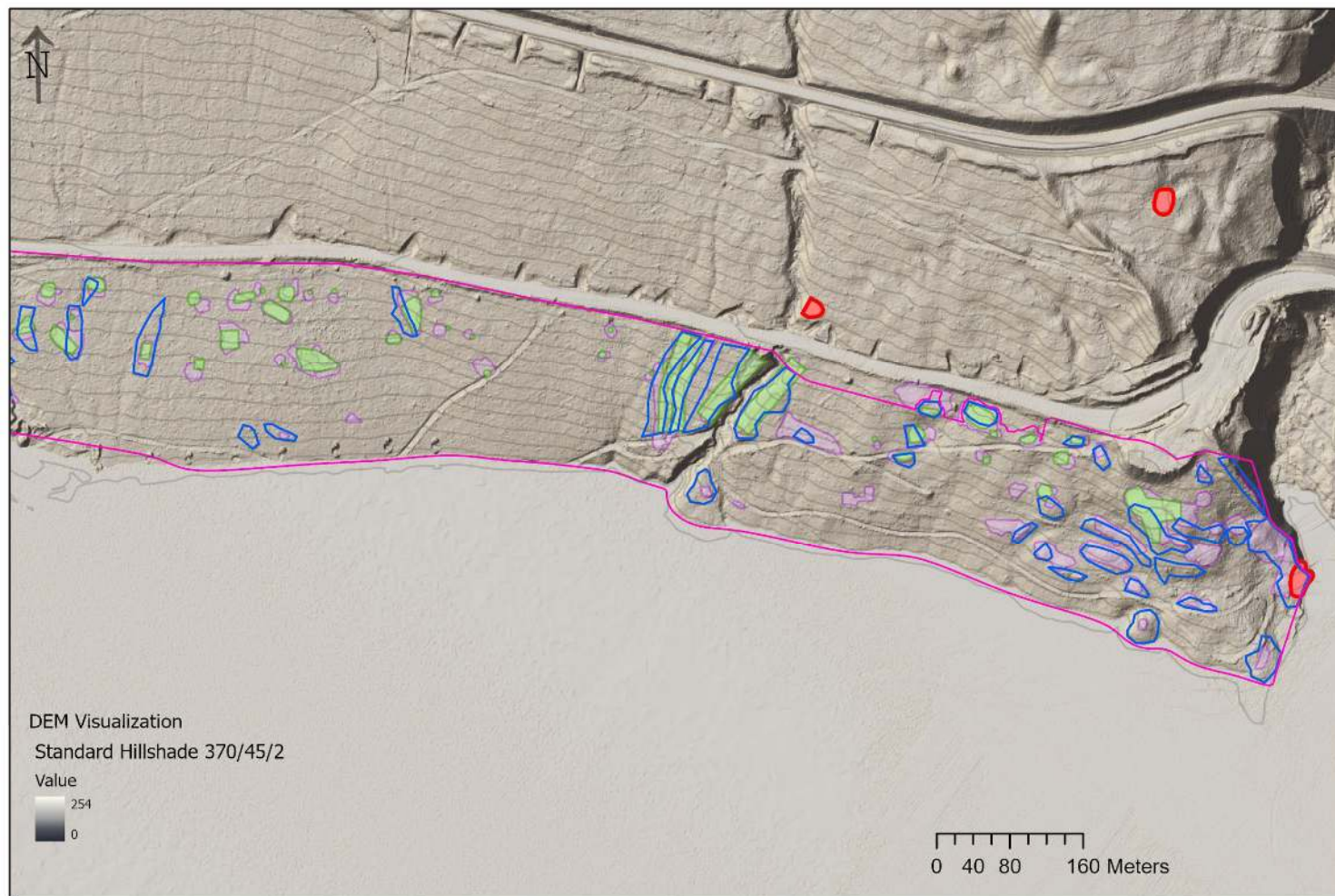
Figure A.1. North tailings test area 1 showing NNTC AOI polygons (green), NNTC STA polygons (purple), MFE Review 2 AOIs (blue), recorded archaeological sites (red), examples of false positives and missed target features Data Source: 2014 LiDAR DEM property of Teck Resources; Standard Hillshade (Azimuth=270; Angle=45; z-factor=2); ArcGIS Pro produced 2.5 m contour lines
