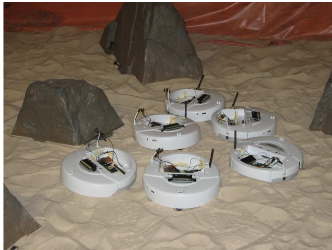
Fig. 1. The multi-robot network. This network is used in the pre-Antarctic stages of this project. Its mobility and sensor abilities approximate the Antarctic network sufficiently to assemble and deploy formations using the same automatic tools.
