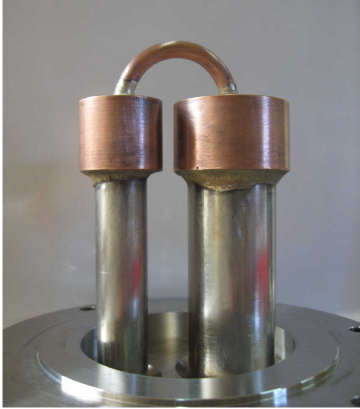
Figure 3. Cold head of the first stage PTC
