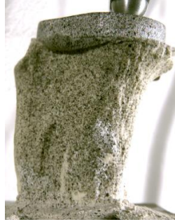
Figure 3.4: Captured image of bone-cement-aluminum by camera in compressive oscillating load.
