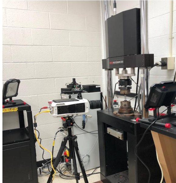
Figure C.4: The set up the experiment of a piece of Aluminum in compression.
