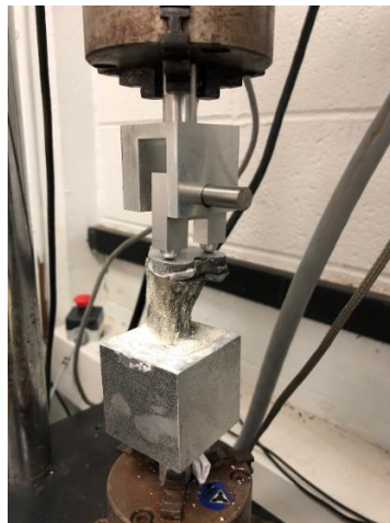
Figure 3.2: Set up the sample in the Test Resources machine to apply the compressive oscillating load.
