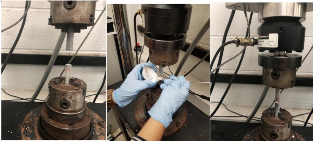
Figure 2.2: (left) two aluminum rods placed perpendicularly at a distance apart; (center) inserting the cement between two aluminum; (right) compression of the cement
