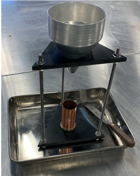
Figure 2- 6 shows the setup for uncompact void content apparatus
