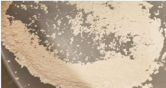
Figure 1- 3 shows an example of fines materials retained on a pan
