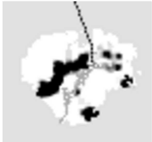
Fig. 8. The map, trajectory and plan resulting from an experiment using only a planner. Because the planner is too optimistic for the configuration space of the physical robot, the robot collides with obstacles while trying to navigate through the narrow opening.
