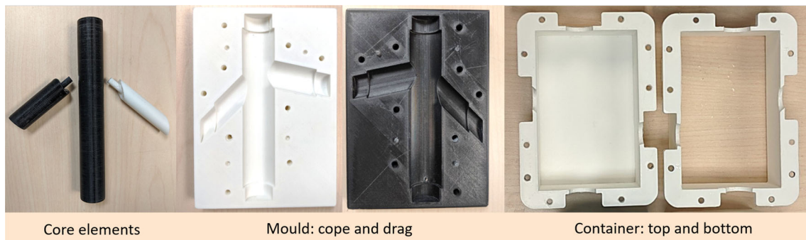
Fig. 5 Solid parts of phantom, 3D-printed in poly-lactic acid (PLA) plastic material. From left to right: disassembled core elements with collinear cylindrical joints; cope and drag for the mould; bottom and top half of the custom container
