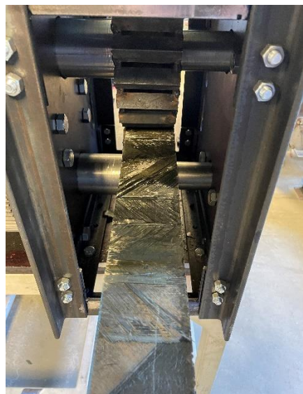
Figure 12: Partially Delaminated Input
